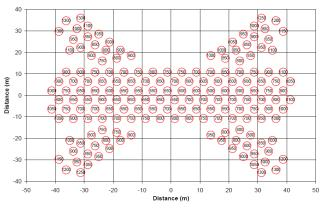
Figure 8. Computed Pile Head Vertical Stiffness Values (MN/m)
