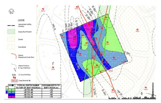
Figure 3. Inferred Contours of Top of Soft Rock
