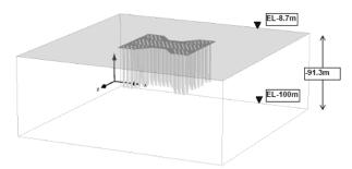
Figure 9. Schematic of PLAXIS 3D Model
