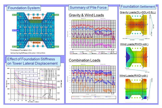
Figure 12. Summary of Foundation Analysis from Midas Program; Soil-Structure Interaction
